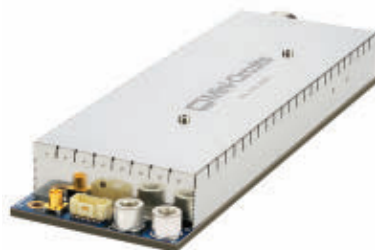
5. To boost signal levels in the 2.4- to 2.5-GHz ISM band, this coaxial SSPA from Mini-Circuits employs Si LDMOS devices to generate a 300-W pulse and CW output power. Mini-Circuits
