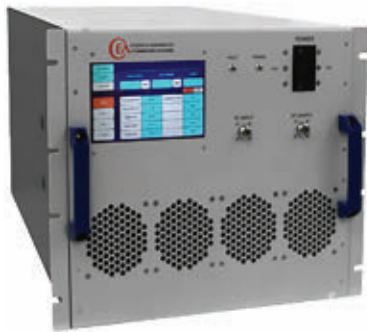
3. Depending on the choice of gain (60 or 63 dB), Exodus's PA provides 1- or 2-kW output power from 1 to 2 GHz. Exodus Advanced Communications
