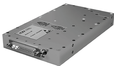
2. Teledyne e2v's MPM combines a TWT and solid-state preamplifier for 125-W output power from 2 to 18 GHz. Teledyne e2v
