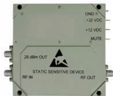
6. Designed for pulsed operation, Mercury's PA delivers as much as 1600-W saturated output power from 1.2 to 1.4 GHz. Mercury Systems
