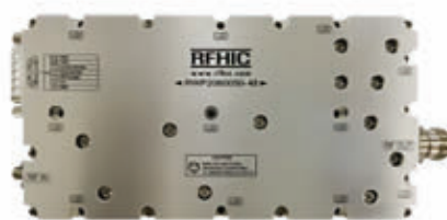
Built using on GaN-on-SiC technology, this SSPA from RFHIC provides 65-W output power from 2 to 6 GHz in a package measuring just 175 \times 90 \times 23 mm. RFHIC
